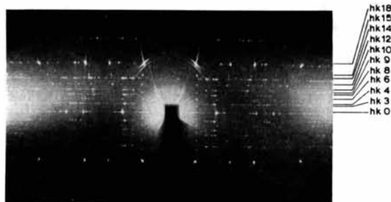
Fig. 1. Oscillation photograph of \text{Cu}_3\text{Si} . The intense layer lines are indicated.
